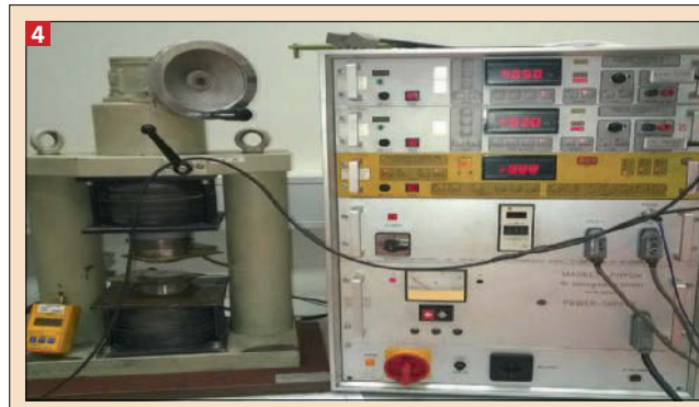
Figure 4: Permagraph of company Steingroever [11].
