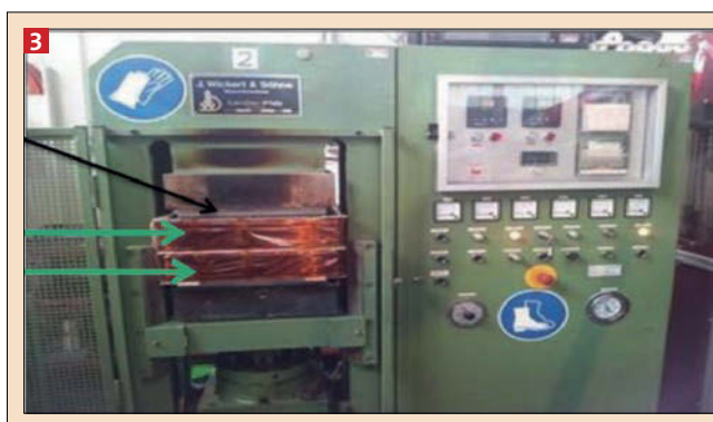
Figure 3: Schematic of the curing setup for the preparation of magnetic-mechanically oriented samples during vulcanisation in an electrical heating press [10].
