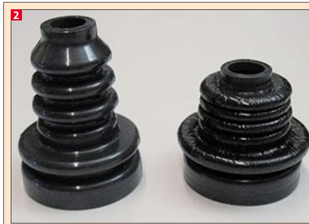
Fig. 2: Standard FKM bellows before and after ageing in pure water at 200 °C.
