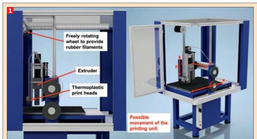
Figure 1: Setup of the new additive manufacturing plant for the AME process
