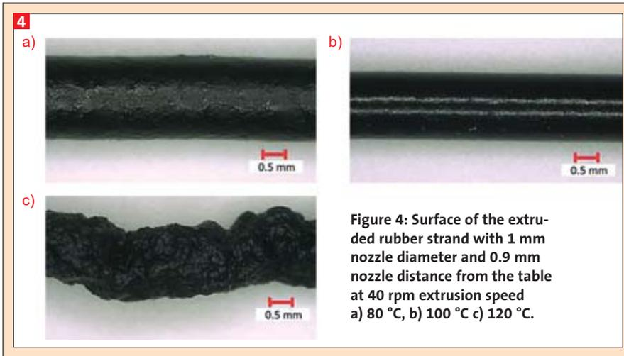
Figure 4: Surface of the extruded rubber strand with 1 mm nozzle diameter and 0.9 mm nozzle distance from the table at 40 rpm extrusion speed a) 80 °C, b) 100 °C c) 120 °C.
