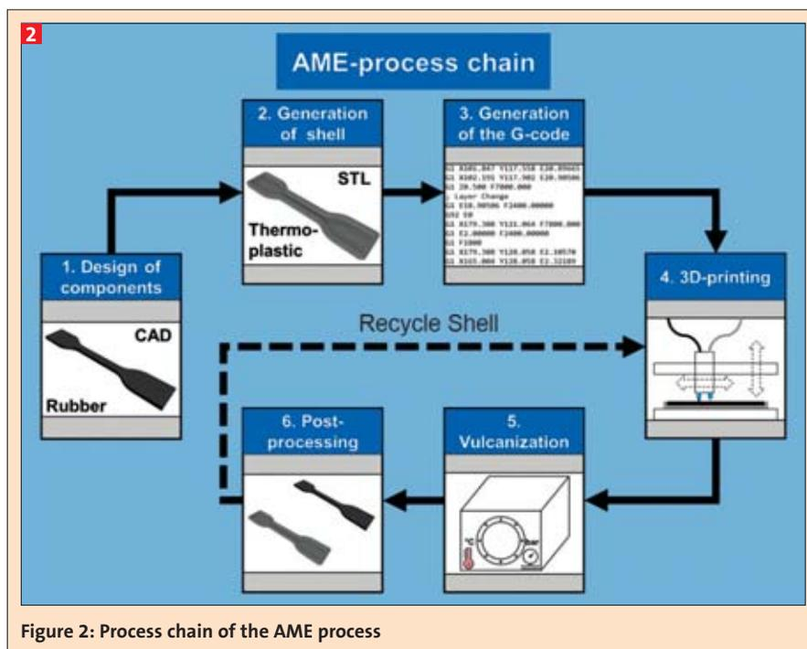
Figure 2: Process chain of the AME process
