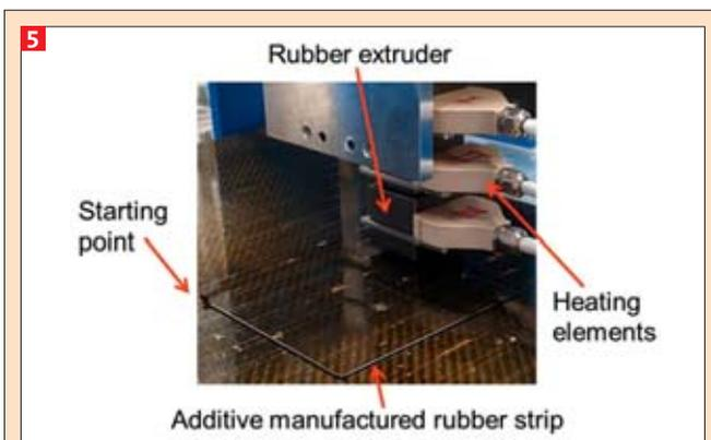
Figure 5: Printed rubber strip at 100 °C, 40 rpm, nozzle diameter 1 mm and nozzle distance to the table 0.9 mm.
