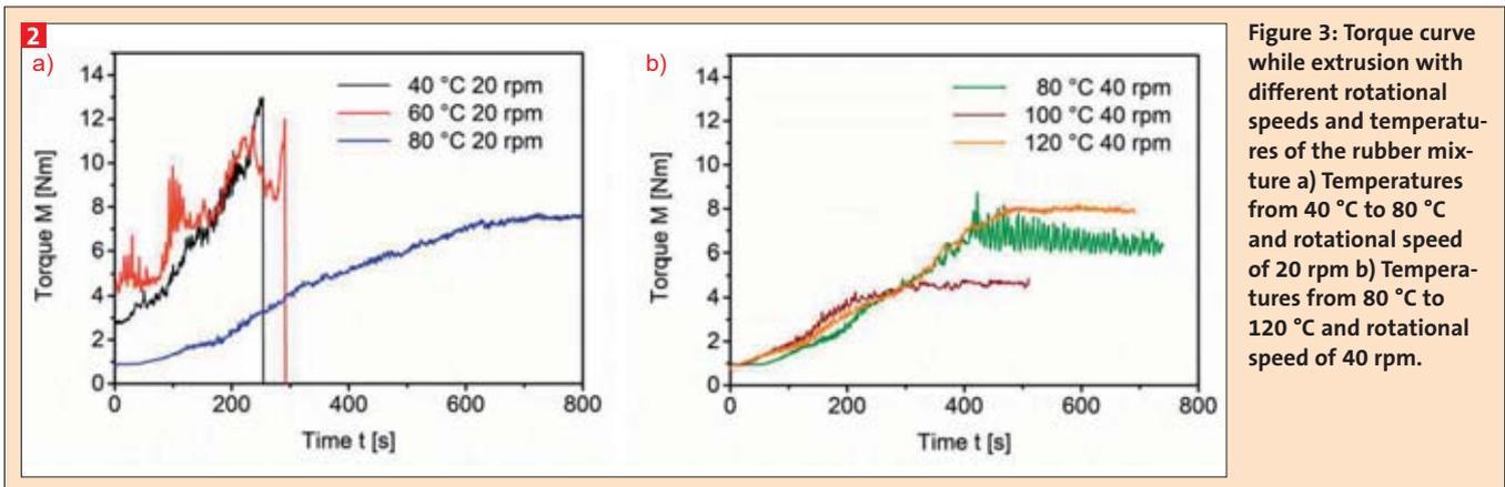
Figure 3: Torque curve while extrusion with different rotational speeds and temperatures of the rubber mixture a) Temperatures from 40 °C to 80 °C and rotational speed of 20 rpm b) Temperatures from 80 °C to 120 °C and rotational speed of 40 rpm.
