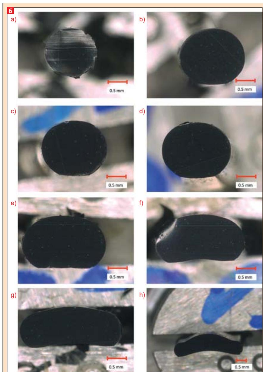
Figure 6: Influence of the nozzle distance from the printing bed a) 2.1 mm b) 1.9 mm c) 1.7 mm d) 1.5 mm e) 1.3 mm f) 1.1 mm g) 0.9 mm h) 0.7 mm.
