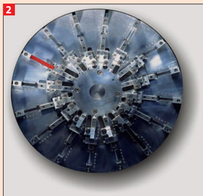
2 Dynamic disk for continuous stretching and release of 16 samples.
