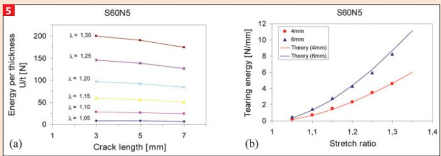
**5** Stored energy obtained with strip samples (SEN-geometry) of the S-SBR with 50 phr N550 divided by the sample thickness  $t$  vs. cut length for various strains (a) and evaluated tearing energy according to Equ. (3) vs. strain (symbols) at various cut lengths, as indicated (b). The lines in (b) are calculated by Equ. (1) with  $\alpha = 2.5$  and  $\alpha = 3.1$  for  $c = 4$  mm and  $6$  mm, respectively
