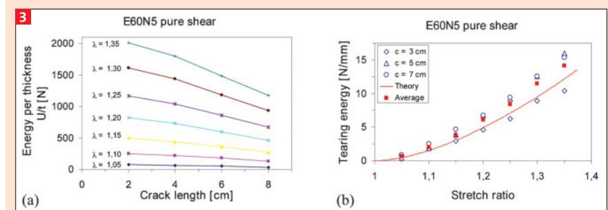
3 Stored energy obtained with pure shear geometry of the EPDM-samples with 50 phr N550 divided by the sample thickness  $t$  vs. cut length for various strains (a) and evaluated tearing energy according to Equ. (3) vs. strain (symbols) at various cut lengths, as indicated (b). The line in (b) is calculated by Equ. (2)
