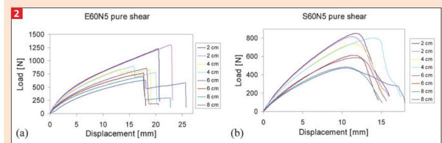
2 Load-displacement curves obtained with pure shear geometry of the EPDM-samples with 50 phr N550 (a) and S-SBR samples with 50 phr N550 (b) at various cut lengths, as indicated
