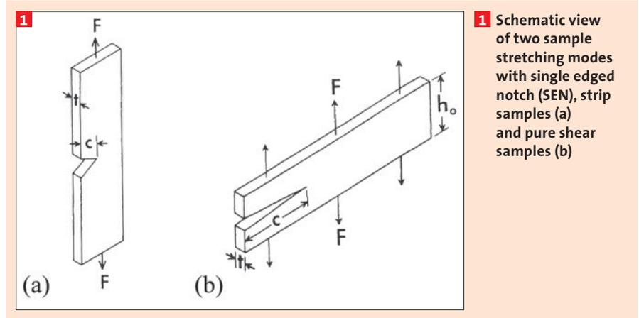
1 Schematic view of two sample stretching modes with single edged notch (SEN), strip samples (a) and pure shear samples (b)
