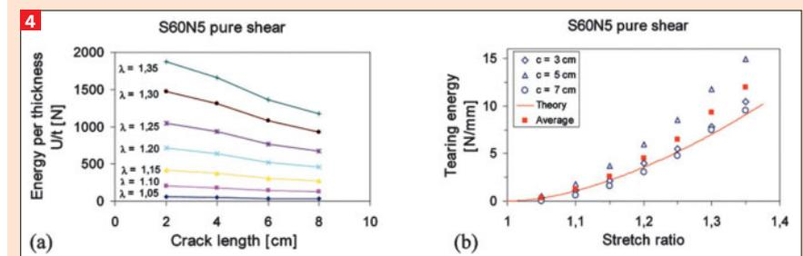
4 Stored energy obtained with pure shear geometry of the S-SBR samples with 50 phr N550 divided by the sample thickness  $t$  vs. cut length for various strains (a) and evaluated tearing energy according to Equ. (3) vs. strain (symbols) at various cut lengths, as indicated (b). The line in (b) is calculated by Equ. (2)
