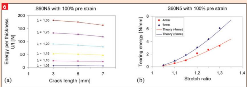
**6** Stored energy obtained with 100% pre-conditioned strip samples (SEN-geometry) of the S-SBR with 50 phr N550 divided by the sample thickness  $t$  vs. cut length for various strains (a) and evaluated tearing energy according to Equ. (3) vs. strain (symbols) at various cut lengths, as indicated (b). The lines are calculated by Equ. (1) with  $\alpha = 2.0$  and  $\alpha = 2.3$  for  $c = 4$  mm and  $6$  mm, respectively
